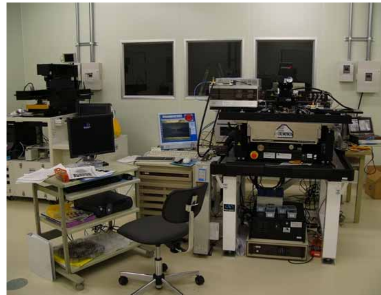
RF measurement system; 8 inch wafer, 40 GHz
